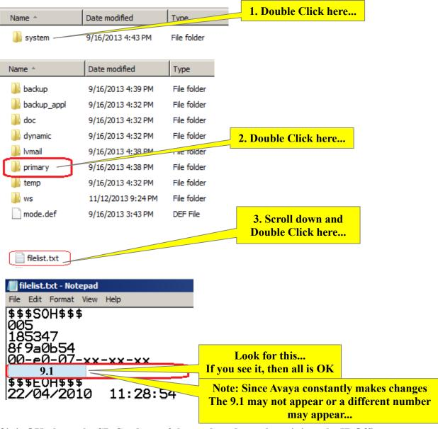
If it is OK, then take SD Card out of the card reader and put it into the IP Office. It will keep the original Feature Key number but it will be a Release 9.1 SD Card. If the SD Card did not upgrade, do not put it in the KSU.
